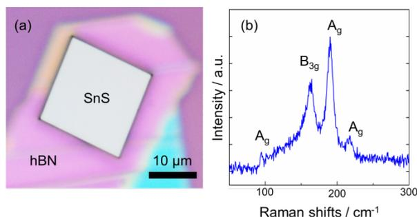
Figure 3. (a) SnS crystal grown on hBN and (b) its corresponding Raman spectrum registered at 532 nm excitation.
